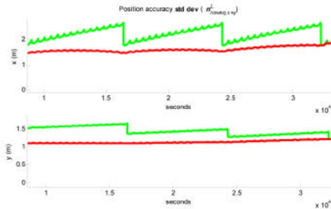
Figure 8 Position accuracy for the Localize mission with GPS fixes every 15<sup>th</sup> line. Line length is 1 km. Green graph: real-time position accuracy ( $1\sigma$ ). Red graph: post-processed position accuracy ( $1\sigma$ ). x and y in local level (L) correspond approximately to North and East direction. A North East aligned mission plan was simulated for simplicity.
