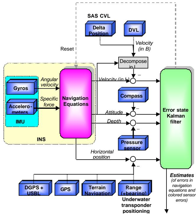
Figure 2 Integrated inertial navigation system structure
