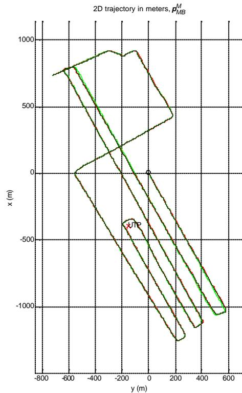
Figure 3 HUGIN 2D trajectory in UTP sea trial. UTP was deployed at  $x = -396$  m,  $y = 151$  m (relative coordinates).
