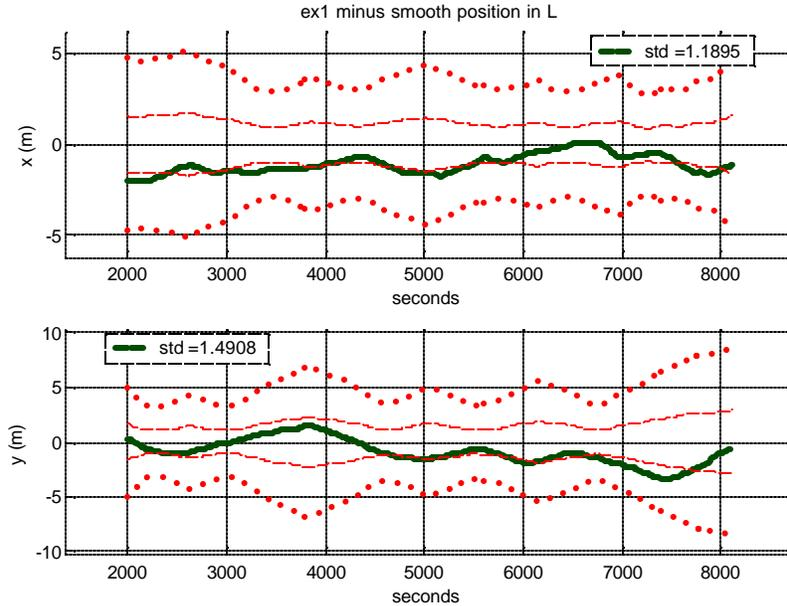
Figure 4 Results from UTP sea trial. Dark graph: difference between UTP post-processed navigation solution and independent DGPSUSBL position estimates. Red dashed and red dotted graphs are  $1\sigma$  and  $3\sigma$  estimated uncertainty of the difference.
