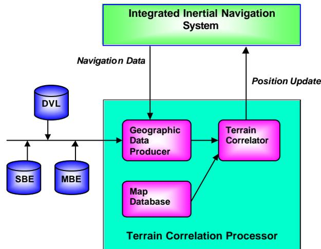
Figure 5 Structure of the HUGIN terrain correlation system
