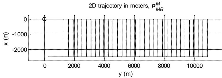
Figure 9 The  $10 \times 10 \text{ km}^2$  Survey area was divided into four areas of  $2.5 \times 10 \text{ km}^2$ . The figure shows simulated mission plan for one of the parts. Position accuracy increases with reduced line lengths. The Explore area was similarly divided into two  $1 \times 10 \text{ km}^2$  areas. Division of the operational area into smaller parts also allows for operation of multiple AUVs and reduced requirements on battery endurance.
