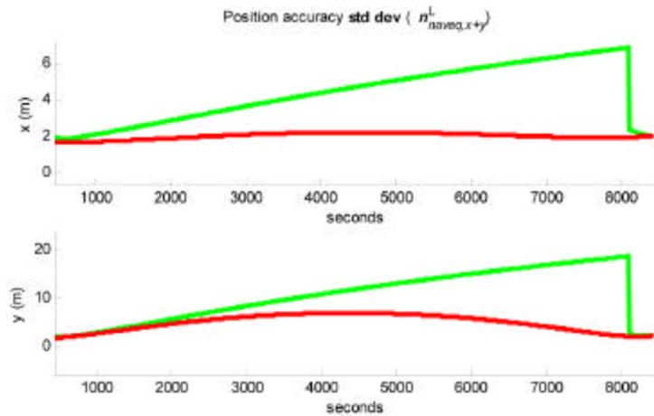
Figure 6 The effect of navigation post-processing when running a straight line with GPS fix after 15 km. Green graph: real-time position accuracy ( $1\sigma$ ). Red graph: post-processed position accuracy ( $1\sigma$ ). x and y in local level (L) corresponds approximately to position uncertainty in across track and along track direction for this particular mission.
