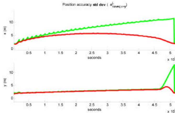
Figure 10 Position accuracy for a  $2.5 \times 10 \text{ km}^2$  part of the Survey area. The mission plan is shown in Figure 9. The AUV surfaced for GPS fixes when entering and exiting the operational area. Green graph: real-time position accuracy ( $1\sigma$ ). Red graph: post-processed position accuracy ( $1\sigma$ ). The increase in y position uncertainty at the end of the mission is due to the 10 km straight-line transit out of the operational area.
