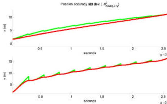
Figure 7 Position accuracy for a 50 km straight-line transit. The AUV makes  $360^\circ$  turns every 5 km to enable estimation and compensation of DVL error and thus increased position accuracy. Since no position measurements are available, the difference between real-time (green graph) and post-processed (red graph) position accuracy is small.
